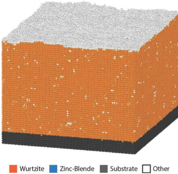
FIG. 18. Simulated as-deposited GaN film grown on a  $(11\bar{2}0)$  GaN surface at an MD temperature of 2800 K ( $T^*/T_m^* = 0.78$ ).
