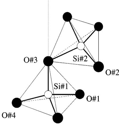
FIG. 11. Schematic representation of two corner-sharing tetrahedra.
